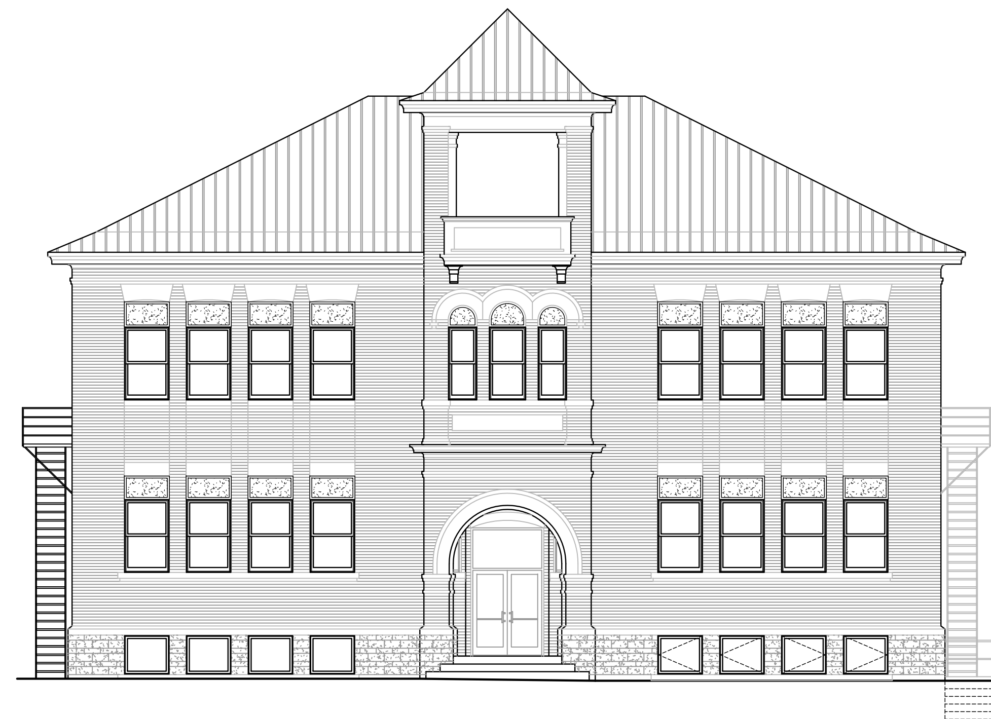
2 PROPOSED FRONT (SOUTH) ELEVATION - MAIN BLDG 1/8" = 1'-0"
