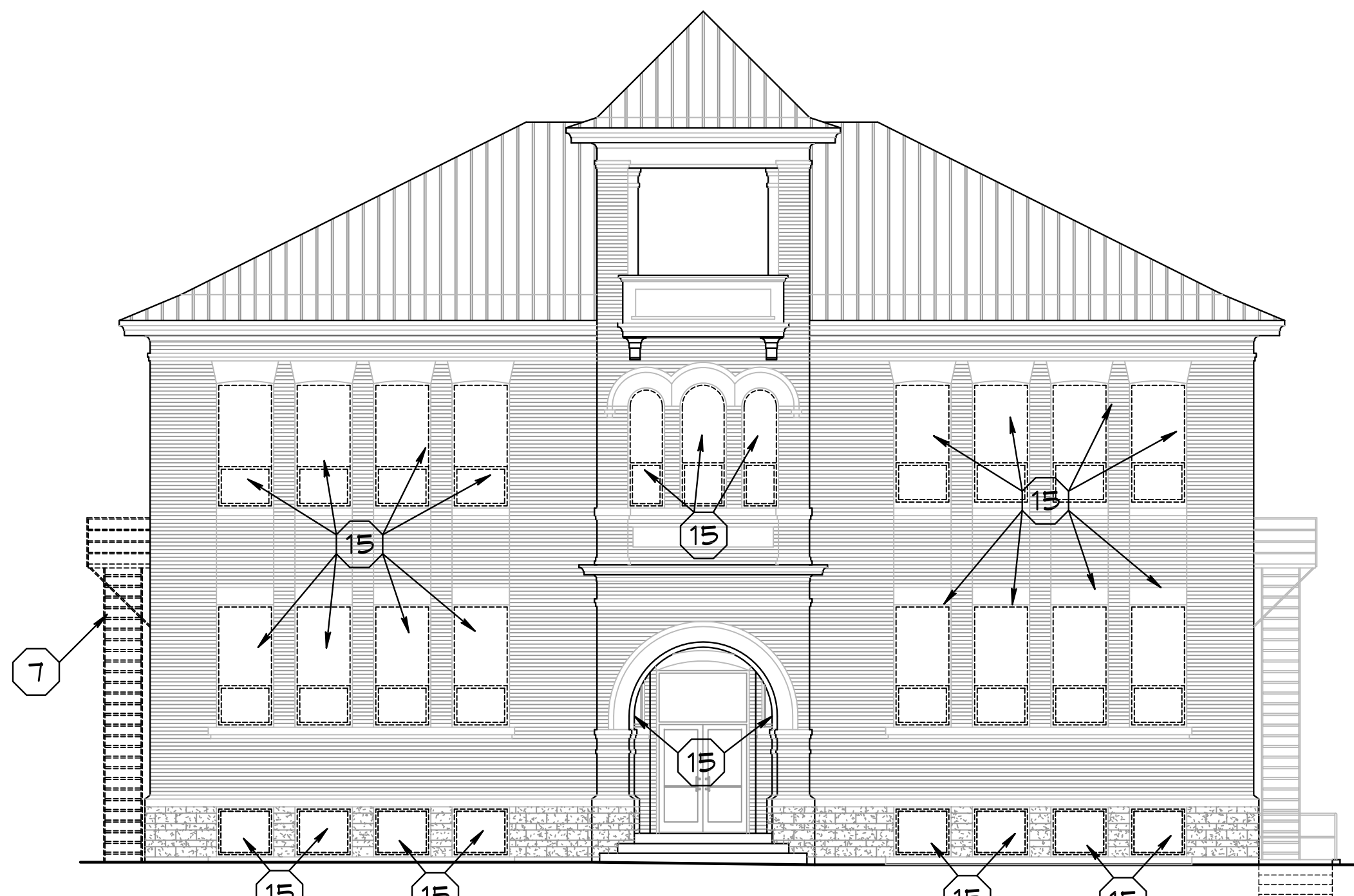
2 DEMO FRONT (SOUTH) ELEVATION - MAIN BLDG 1/8" = 1'-0"
