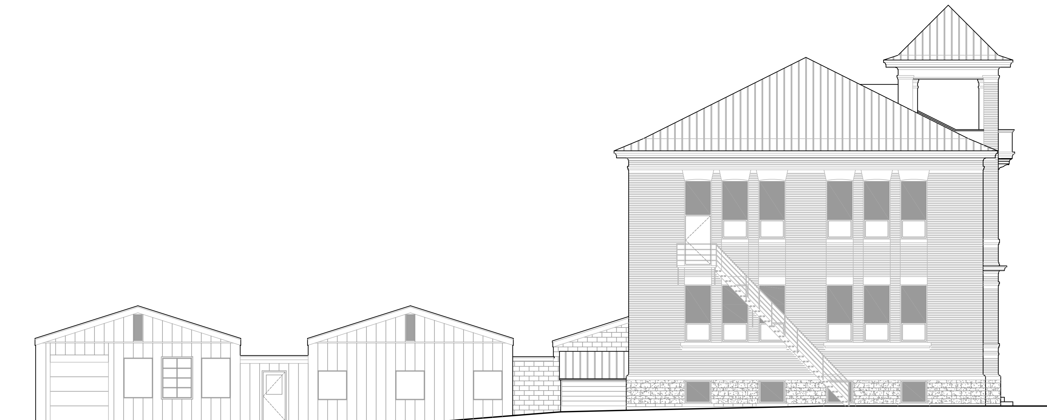
10 EXISTING WEST ELEVATION MAIN & EXTENSION BLDG'S 1/8" = 1'-0"
